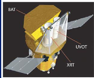
Figure 1: The NASA Gamma-Ray Burst Explorer Mission Swift. It is equipped with an UV/Optical and an X-ray telescope which allow simultaneous Optical/UV to X-ray observations. (Credit: NASA/GSFC)
